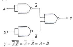
This output equation is equivalent to OR gate.
